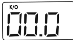
Figure 10-17: Setting the Display’s Keel Offset
