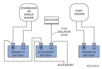
Figure 9-4: Batteries and Isolator
