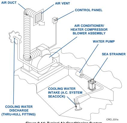
Figure 9-14: Typical Air Conditioning System
