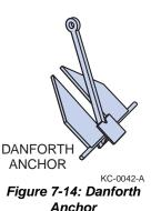
For most applications, anchor line length should be at least six to seven times longer than the depth of the water in which you are anchoring. Always have plenty of additional anchor line on board. If anchoring in tidal waters, consider a rode chain about the length of the boat and increase the total anchor line length to ten times the depth of the water at low tide.
