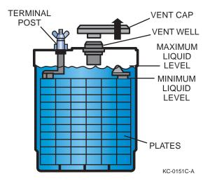
Figure 11-3: Lead-Acid (Wet Cell) Battery
