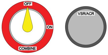
Figure 10-13: Battery Switch with VSR or ACR
