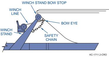
Figure 8-1: Fastening Boat to Trailer
