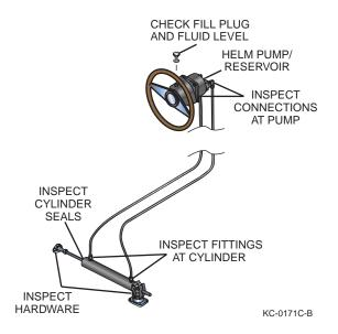
Figure 11-5: Typical Hydraulic Steering System
