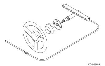
Figure 9-1: Hydraulic Steering System
