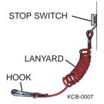
Figure 10-14: Emergency Stop Switch and Lanyard
