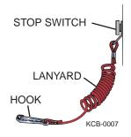
Figure 2-3: Emergency Stop Switch and Lanyard
