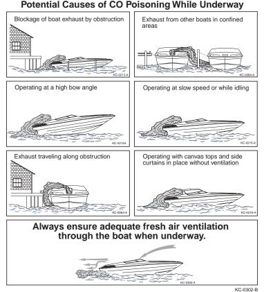
Figure 2-1: Causes of CO Poisoning
