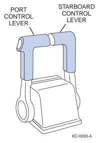
Figure 10-11: Twin-Engine Boats with Single-Lever Controls
