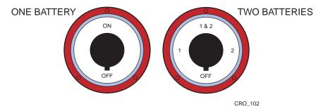
Figure 10-12: Typical Battery Switches
