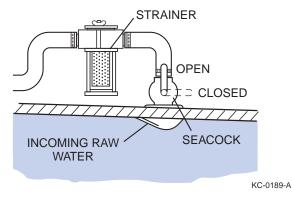
Figure 9-13: Typical Seacock and Strainer
