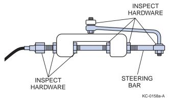
Figure 11-6: Typical Mechanical Outboard Engine Steering Link
