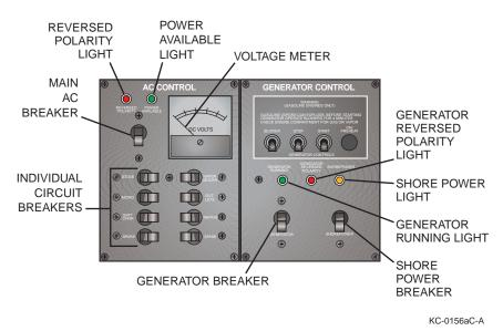
Figure 9-5: Typical AC/Generator Control Panel
