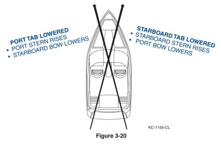
Using trim tabs in conjunction with the power trim will compensate for uneven weight distribution, listing, water conditions and other factors that cause inefficient operation. Remember that trim tabs are trimming the hull while power trim is trimming the engine drive.
