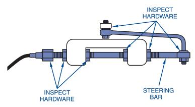
TYPICAL OUTBOARD ENGINE STEERING LINK
